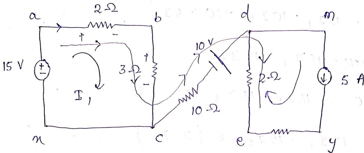
Find the voltage drop between the terminal α and e.
