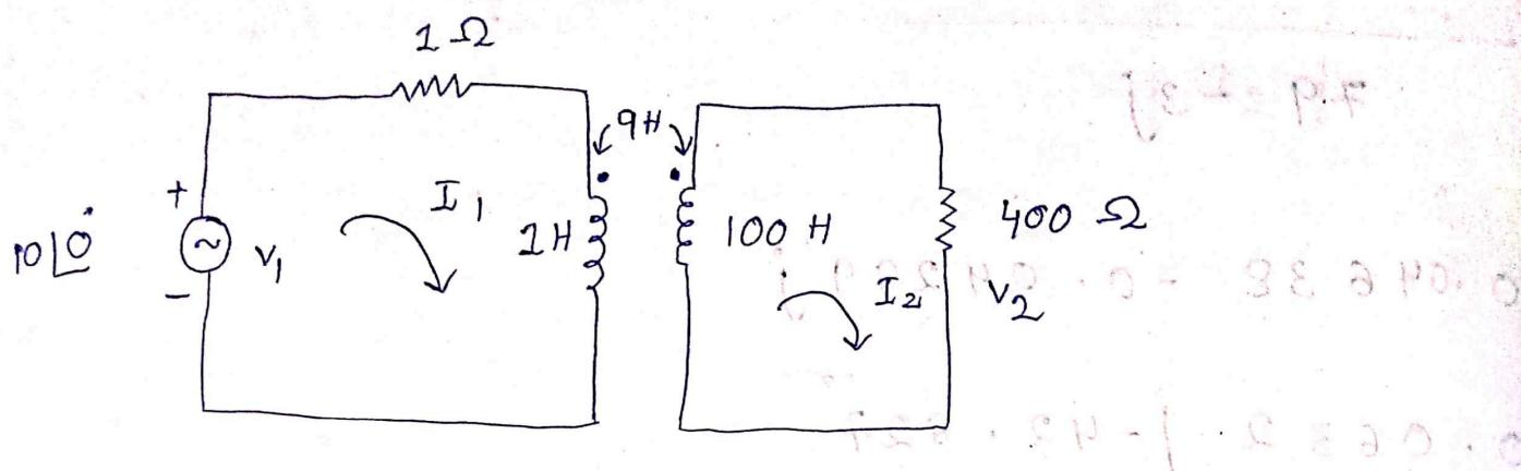
Calculate the ratio of the output voltage across 400  $\Omega$  resistor to the source voltage for the circuit shown in the figure.
