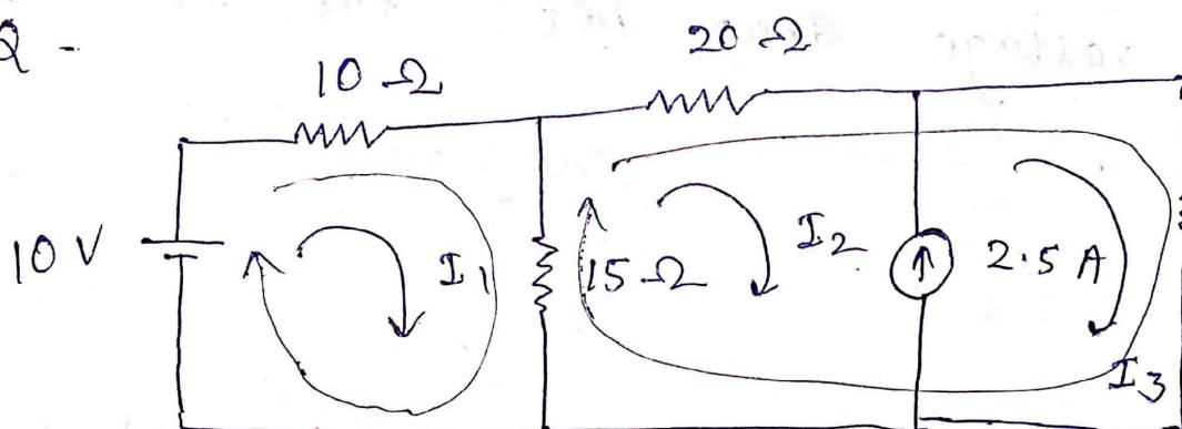
Find the current across  $15\Omega$  resistor using mesh analysis.
