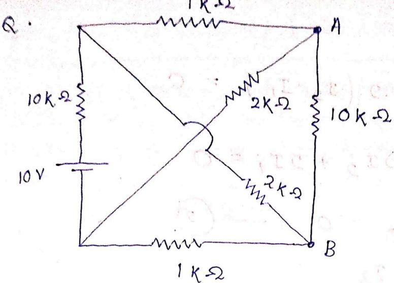
find the voltage across  $10\text{k}\Omega$  resistor at terminal AB as shown in the figure.
