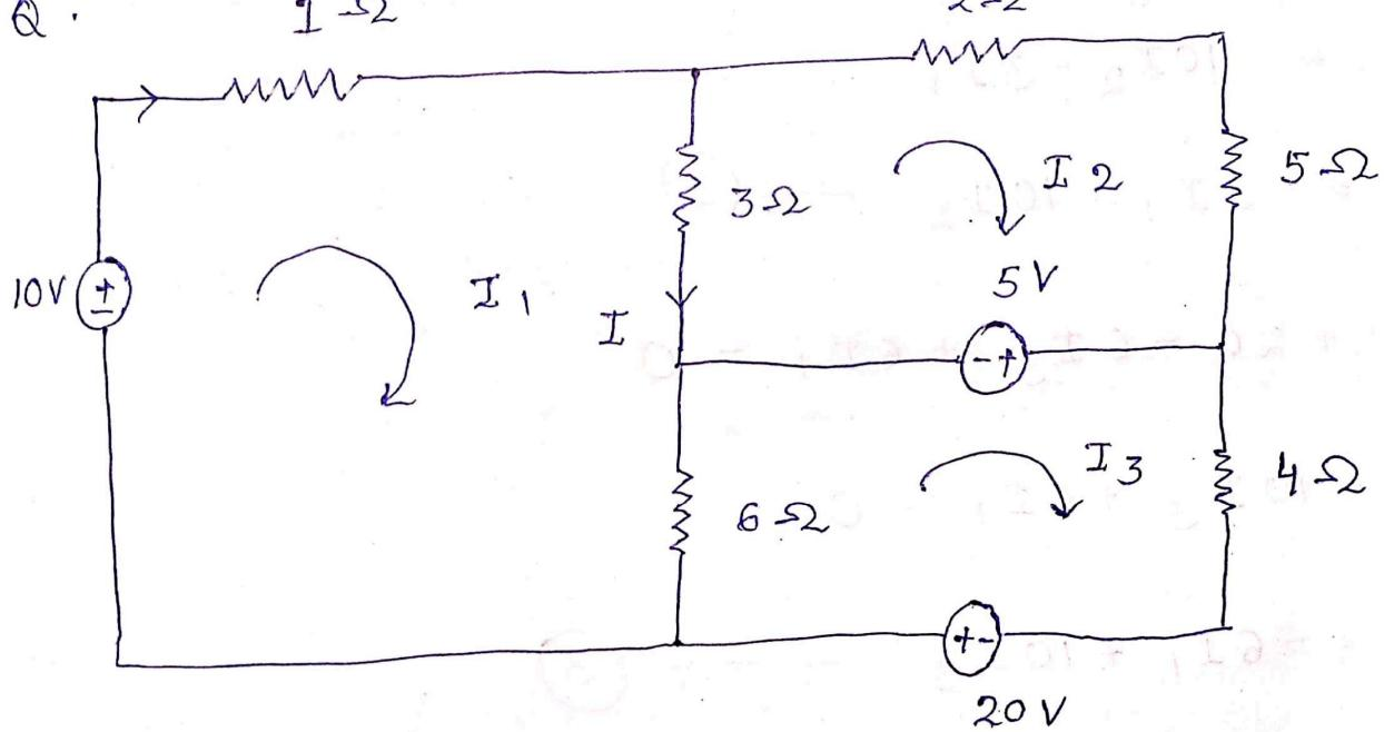
Determine current  $I$  using mesh analysis.
