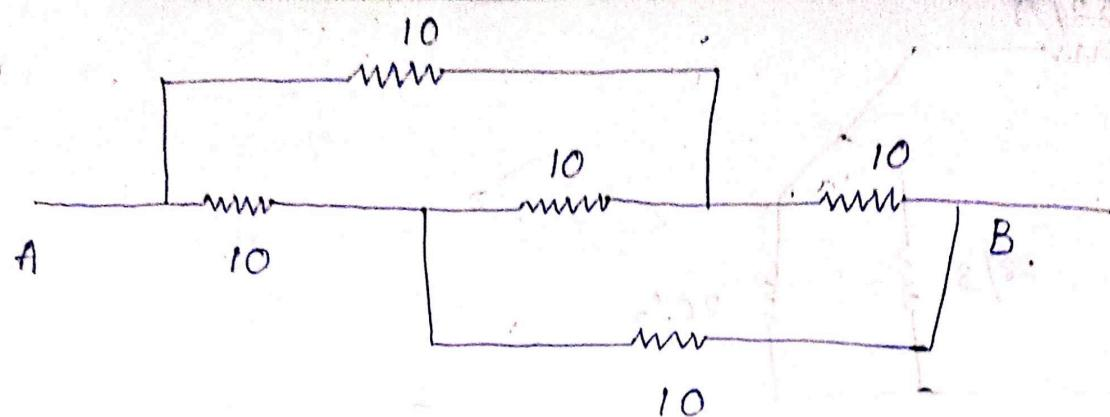
Find the equivalent resistance bet' the terminal A and B.
