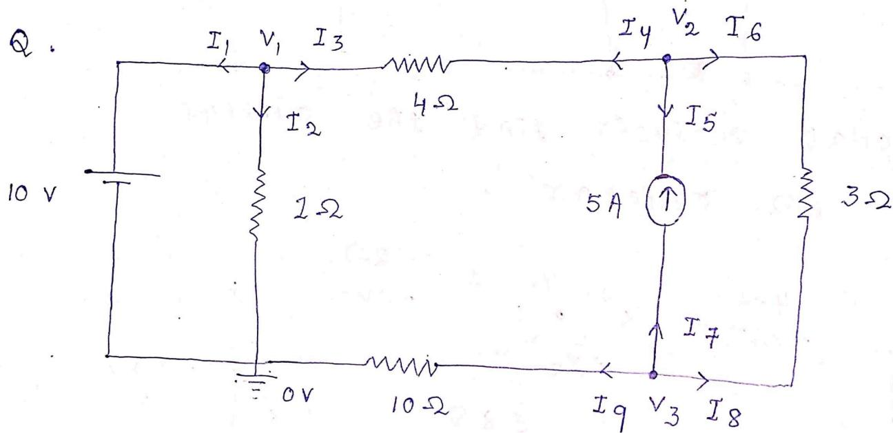
Using nodal analysis find the power dissipation across  $4\Omega$  resistor and current at  $10\Omega$  resistor.
