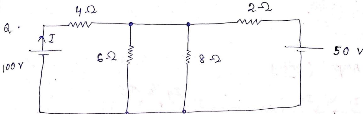
using nodal analysis find the current through 6Ω resistor.
