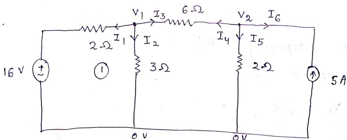
using nodal analysis find the current across 2Ω resistor.
