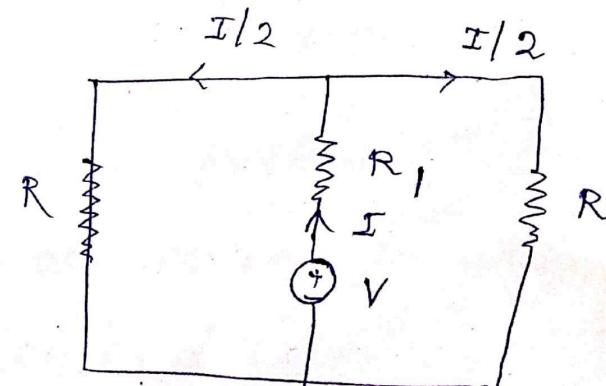
The above figure shows two parallel magnetic circuit ACB and ADB connected across a common magnetic path AB which contains an air gap of length  $l_g$ . The mmf required for the circuit would be the sum of,
