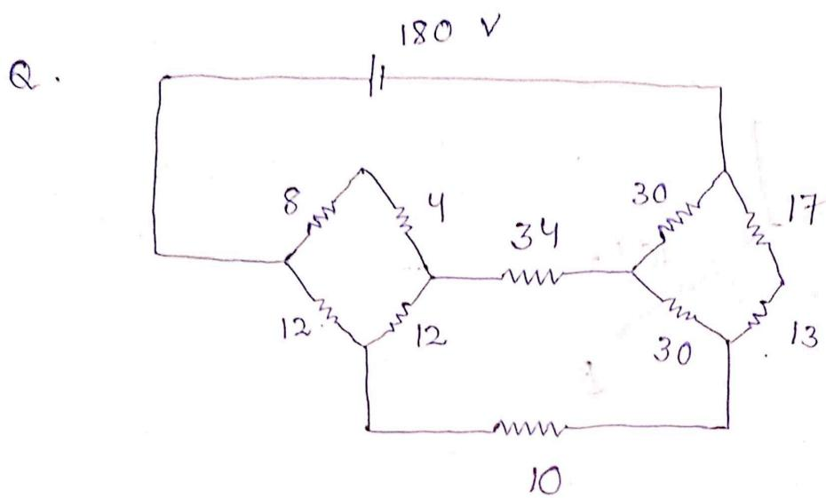
calculate the current through  $10\Omega$  resistor.
